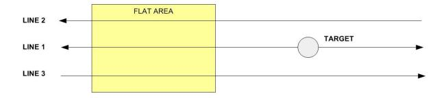
There are three lines, the centre line runs directly over the feature and is sailed twice. The distance between the lines should be about equal to the water depth. If the survey vessel is crabbing the line width needs to be adjusted to ensure the swaths from lines 2 and 3 (runs 3 and 4) overlap at 45 degrees from nadir.
