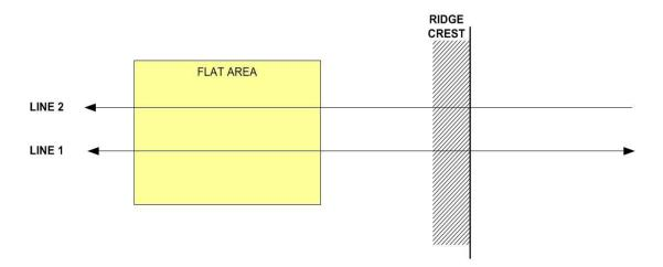
There are two lines, line 1 is run twice. The distance between the lines should be about twice the water depth. If the survey vessel is crabbing, the line width needs to be adjusted to ensure the swaths from each line overlap at 45 degrees from nadir.
